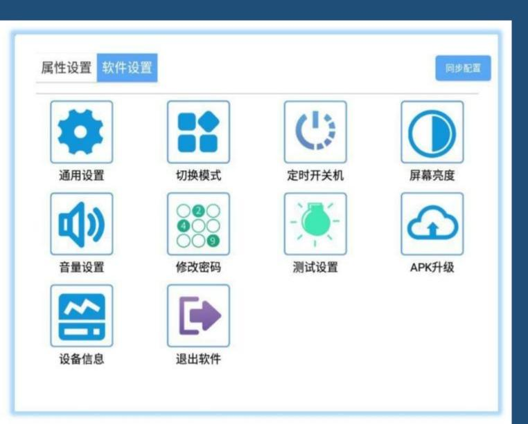
Software Settings Interface :1. General Settings 2. Switching Mode 3. timing switch 4. screen brightness 5. Volume Settings 6. Change Password 7. test settings 2.APK upgrade 9. equipment information 10. Exit software
